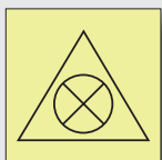
Remote ventilation shutoff PV 6078 JJ
