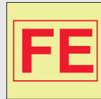
Locker with fireman's outfit PV 6067 JJ
